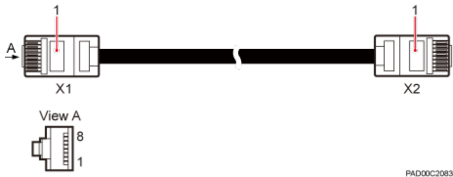
Figure 1-11 Appearance of an Ethernet cable
